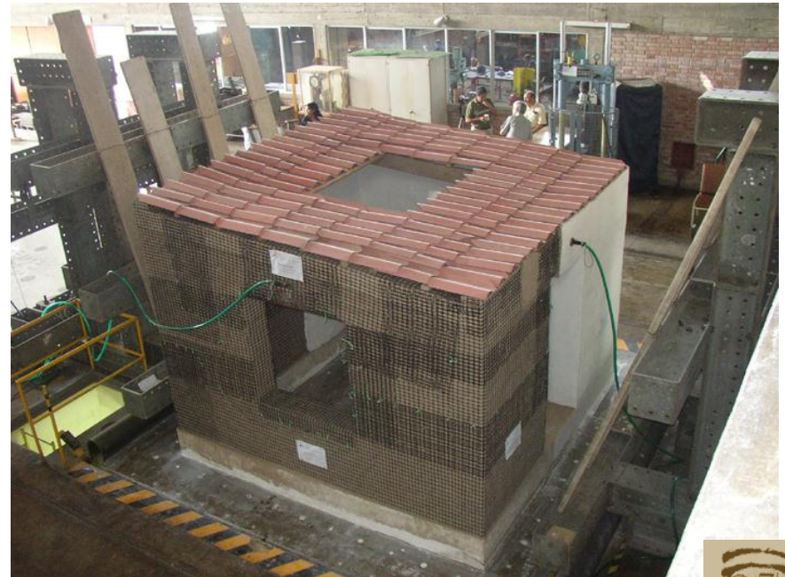
External geomesh reinforcement
