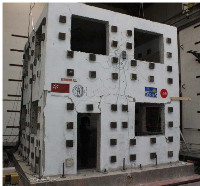
Cracking in rendering around openings and corners
