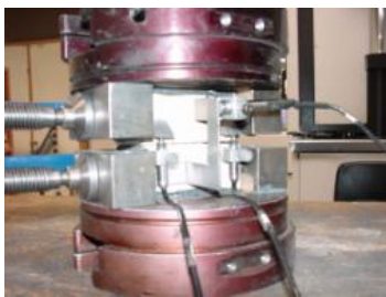
Shear testing of stone joints
