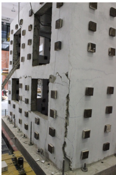
Cracking in rendering around openings and corners
