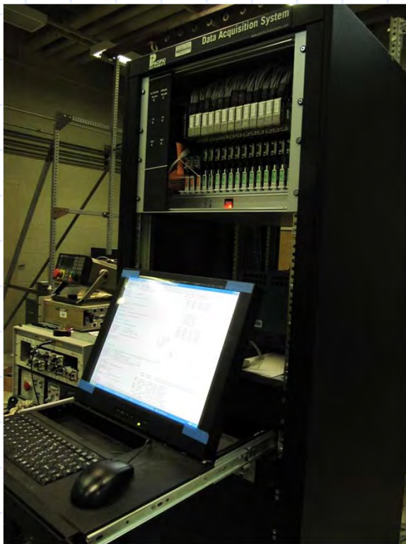
Digital signal processor (DSP) I/O module of Pacific Instruments (PI) DAQ system
